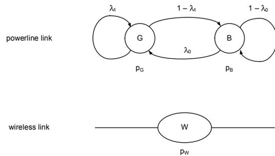
Figure 1: Link models: Gilbert-Elliott Markov model for powerline link (top), and single-state model for wireless link (bottom).
